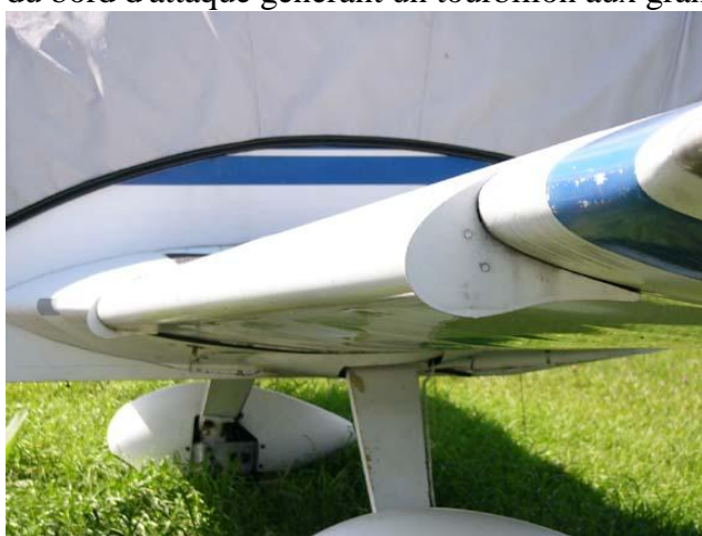
A drooped leading edge cuff installed on an American Aviation AA-1 Yankee as part of a NASA experiment
